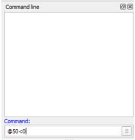
Command line is used for inputs such as Length, Angle, Points
