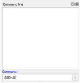
Command-line is used for inputs such as Length, Angle, Points, and can be input the same after the particular command is activated.
