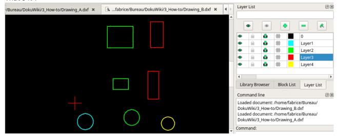
Note that LibreCAD moved the green rectangles of layer 2 in drawing A to the same layer2 in drawing B: so the green rectangles and circles now have the same layer.
