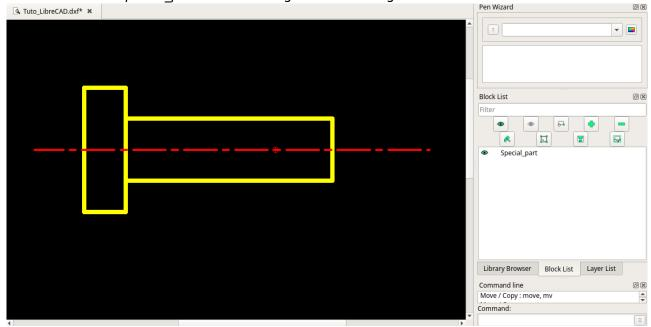
Now, we can insert this block as many times as we want in the current drawing at different locations with different orientations and scales.
