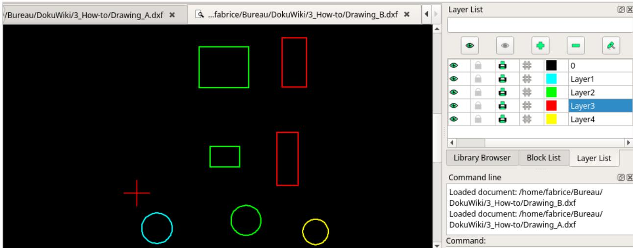
Note that LibreCAD moved the green rectangles of layer 2 in drawing A to the same layer2 in drawing B : so the green rectangles and circles now have the same layer.
