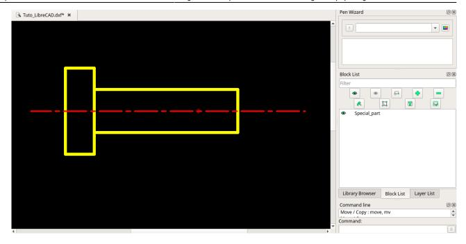
Now, we can insert this block as many times as we want in the current drawing at different locations with different orientations and scales.
