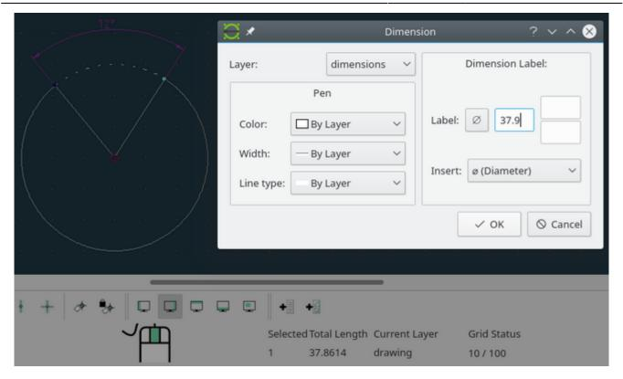
**Hint:** you can find the centre of an arc with the **Dimension: Radial** tool; you can even use two radial dimensions as temporary construction lines from which to create the angular dimension.
