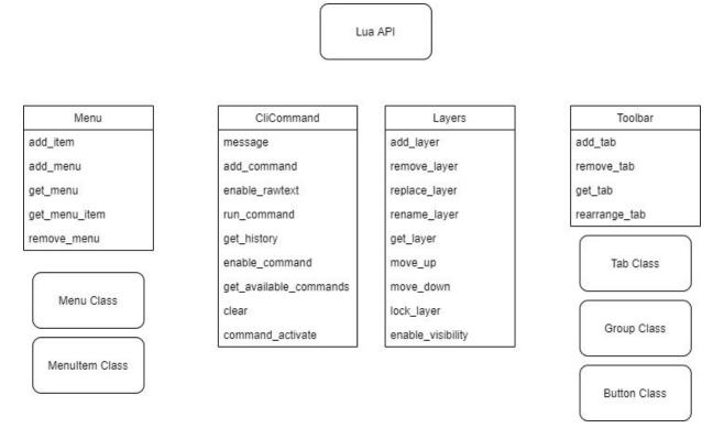
MenuItem class is for the items in a menu(Open, Save as etc.) which are contained in a Menu class (like File, Create etc). The specification for this class is shown in the diagram below.
