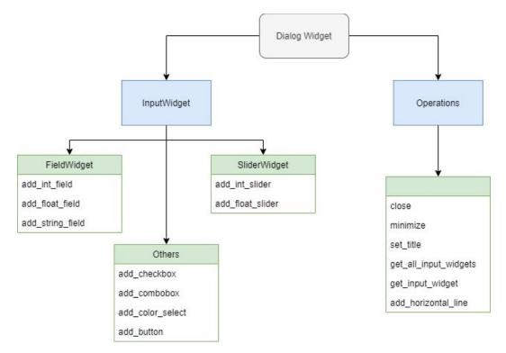
The InputWidget parent class would hold a list of callbacks so that each GUI element can be associated with more than one callback.
